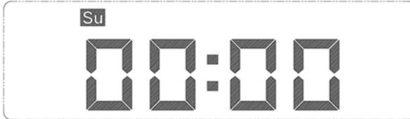
2.2 Press “SET” to set up the clock time (enter Clock-setting mode and display SET and CLK icon). Time and week will start blinking. Press “Hr”, “Min” or “Wk” to set the correct time and week day. The display value will increase by “1” with each press, and the number will change rapidly if user holds the button. The clock will be set and display will become steady (SET and CLK disappear) if there is no key input for one minute (idling or no action).
